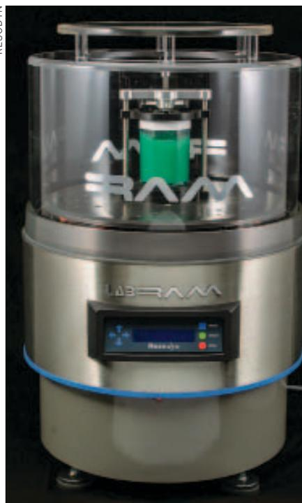
*Combining pharmaceutical compounds in a resonant acoustic mixer like this one forms cocrystals in multigram quantities.*
